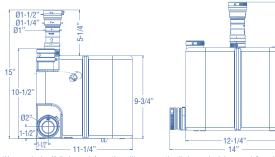
\*Measured using 1" discharge, Information will vary once the discharge size is increased. Consult with factory,
