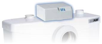
The Sanialarm has a level pressure switch that triggers an alarm fixed on the top of the unit if the volume of water exceeds the maximum allowed level. The alarm emits a continuous 80 dB warning sound until it is switched off or the problem is rectified. The Sanialarm is battery operated and can be installed on most Saniflo macerating units and drain water pumps.
