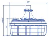
**Discharge pipe diameter:** 2" or 4" Power/Amperage: 220-240V / 60 Hz / 12 A HP: 2 X 1.5 HP Temperature: 158°F Max.
